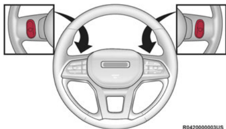
Remote Sound System Controls
